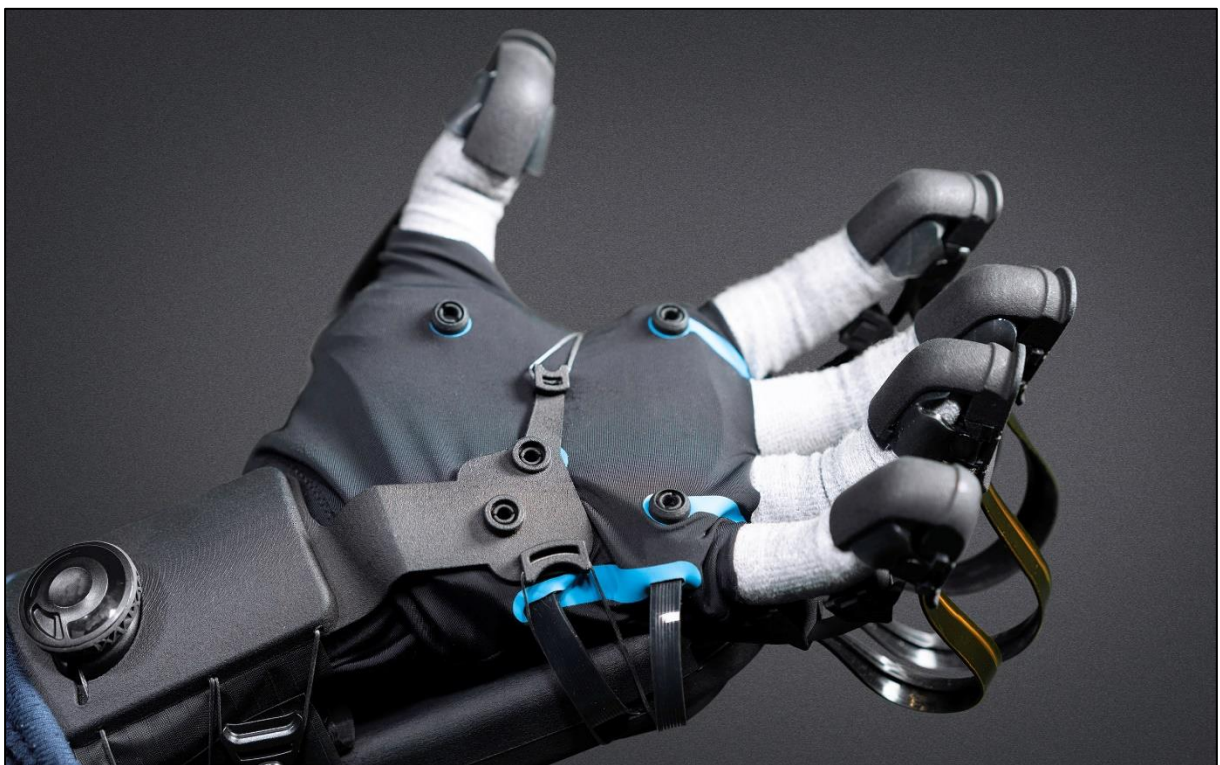
Fig. 15: Glove which allows haptic feedback in VR-experiences [64]. Feedback points make shapes, textures and motions of virtual objects tangible while an exoskeleton provides resistive force. At the same time, magnetic motion tracking allows interactions with the environment.
